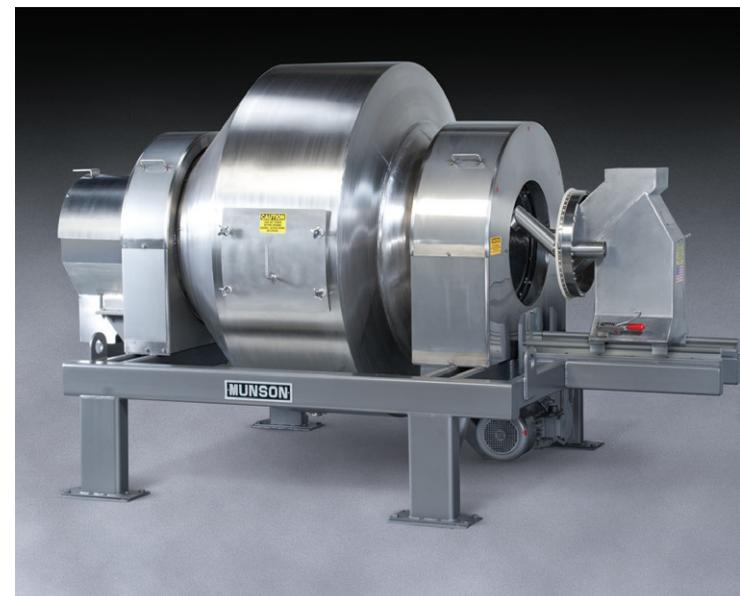
With a batch capacity of 140 cu ft, the rotary batch mixer at NuTech Biosciences has doubled output of nutritional feed supplements.
