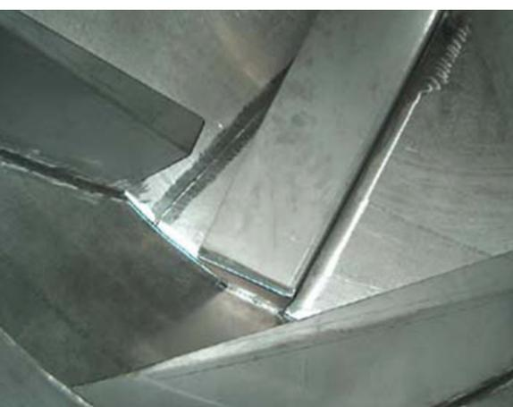
Internal mixing flights produce a tumble-turn-cut-fold mixing action that achieves uniform blends.
